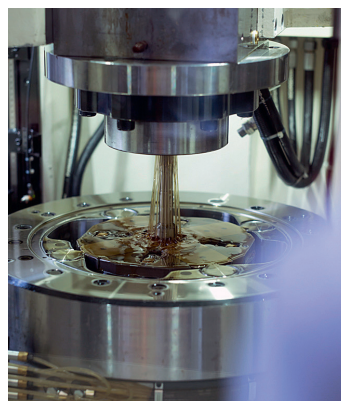
The axial forming process of an external spline profile
