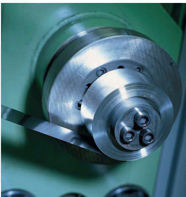
The stripwinding process
